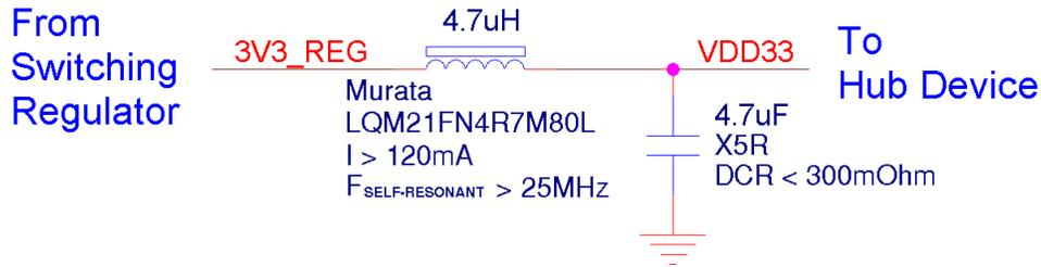
Figure 2.2 Example Switching Regulator Noise Filter
