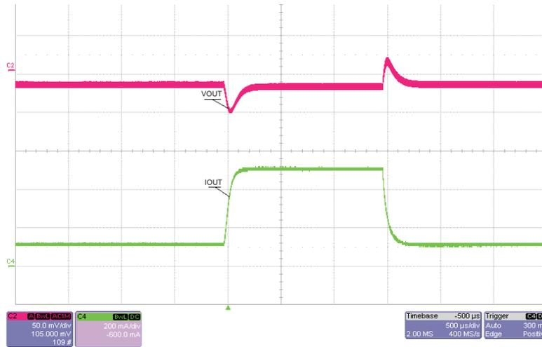
Figure 5. Load Step 100 mA to 500 mA
