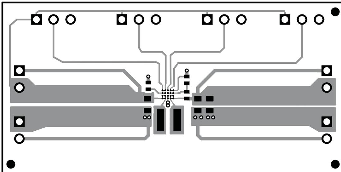
Figure 8. Top Layer Routing
