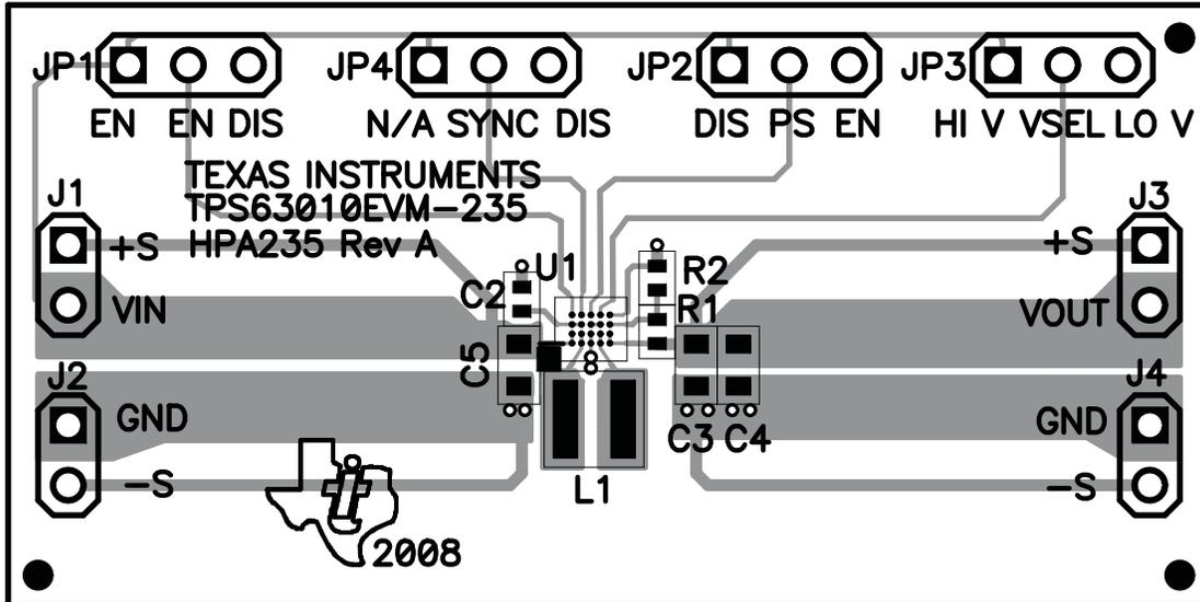
Figure 7. Assembly Layer
