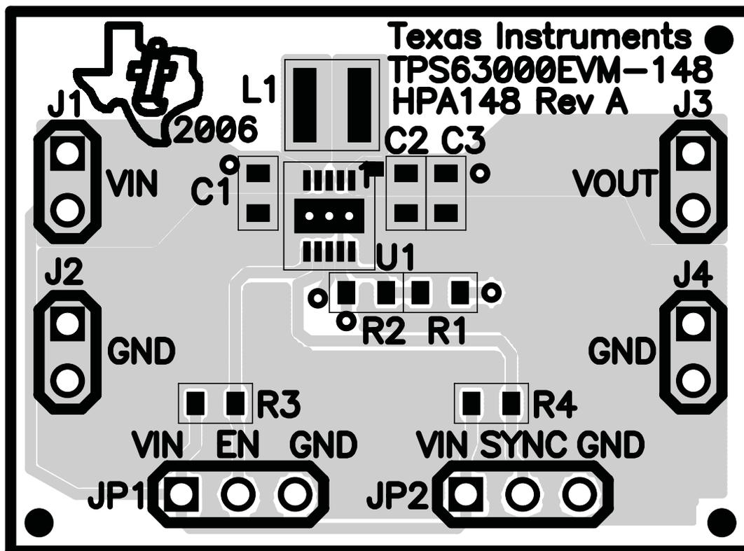
Figure 6. Assembly Layer
