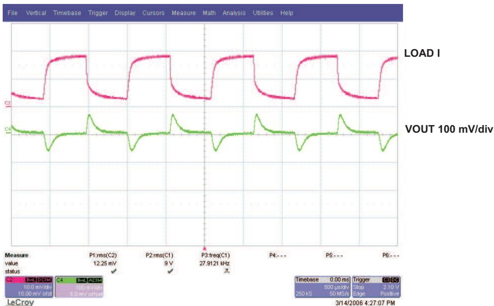
Figure 5. Load Step 100 mA to 500 mA
