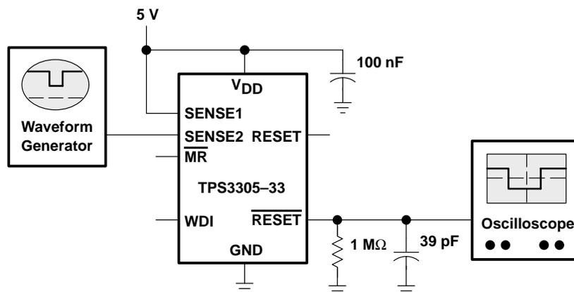
**Figure 10. Circuit for Measuring the SVS Reaction to a Voltage Drop**
