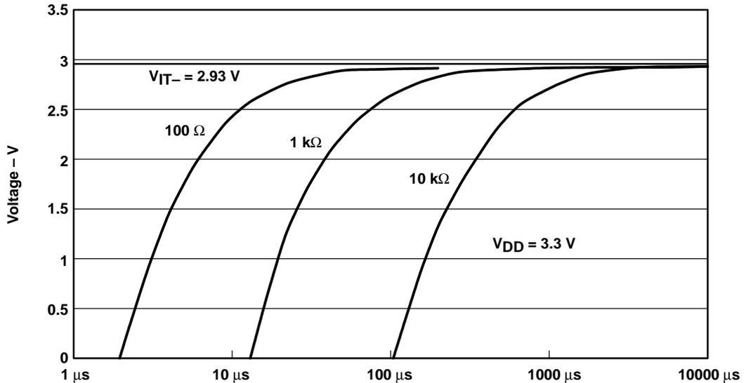
Figure 18. Breakdown Voltage Over Pulse Width With a Low-Pass Filter at SENSE2
