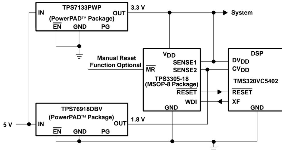
The necessary decoupling capacitors are not shown to increase the clearness of the figure.
