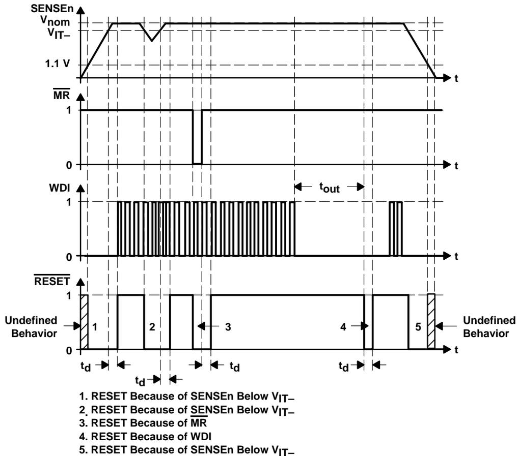
Figure 7. Basic Timing of the TPS330x
