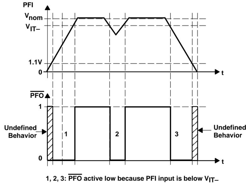
**Figure 8. PFI and  $\overline{\text{PFO}}$  Basic Timing**
