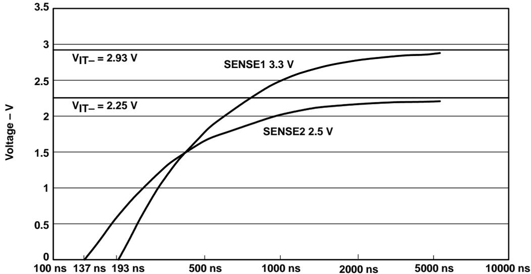
Figure 15. Breakdown Voltage Over Pulse Width (TPS3305-25, TPS3307-25)
