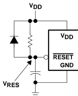
**Figure 1. A Simple Reset Solution**
