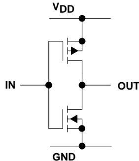
**Figure 34. Conventional Totem Pole Output Stage**
