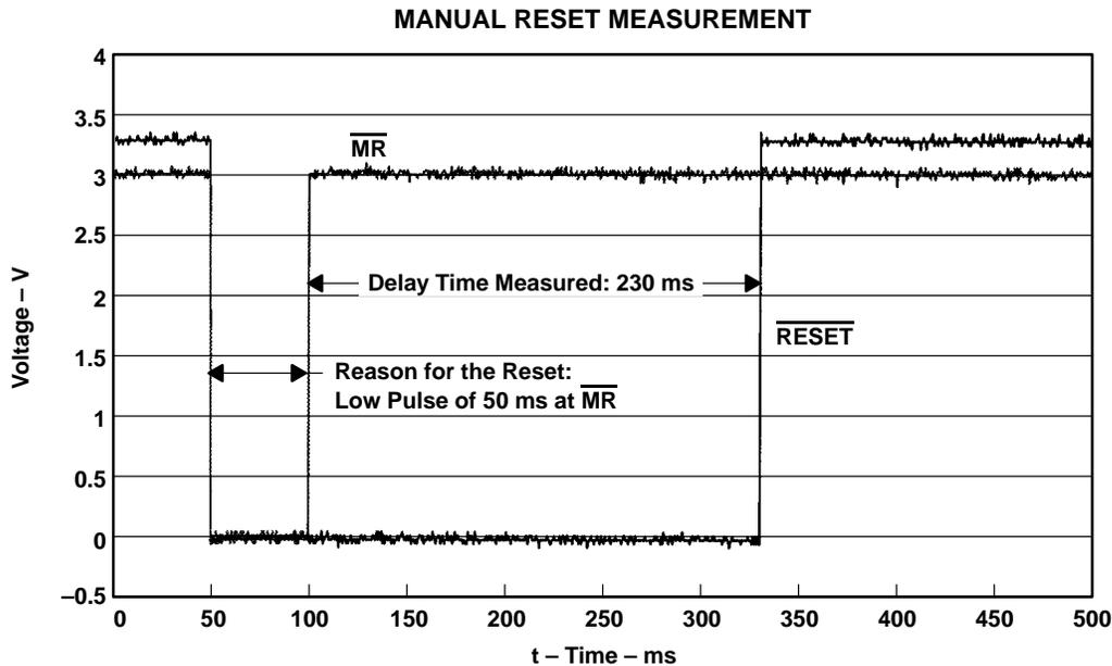
Figure 19. Measurement of a Reset Pulse Triggered by Manual Reset
