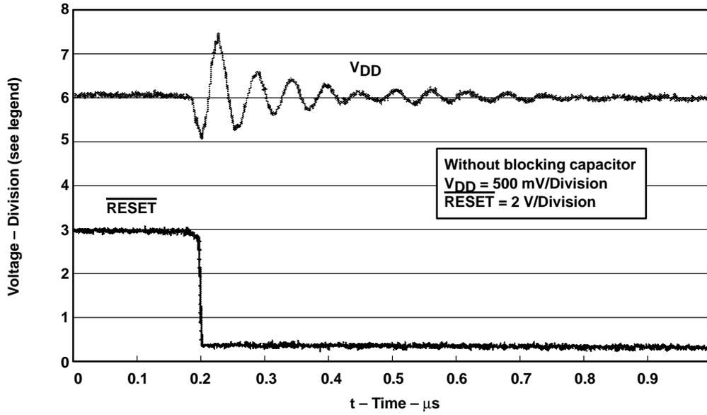
**Figure 32.  $V_{DD}$  – Line of TPS3305–33 Without a Capacitor**
