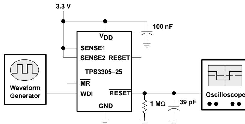
Figure 21. Measurement Circuit for Testing the Watchdog
