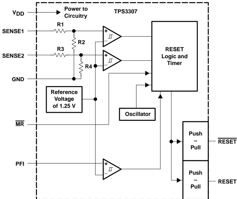
Figure 6. Block Diagram of the TPS3307
