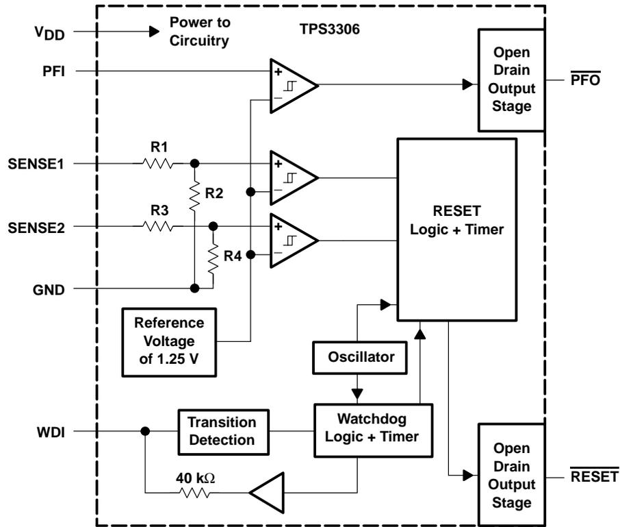
Figure 5. Block Diagram of the TPS3306
