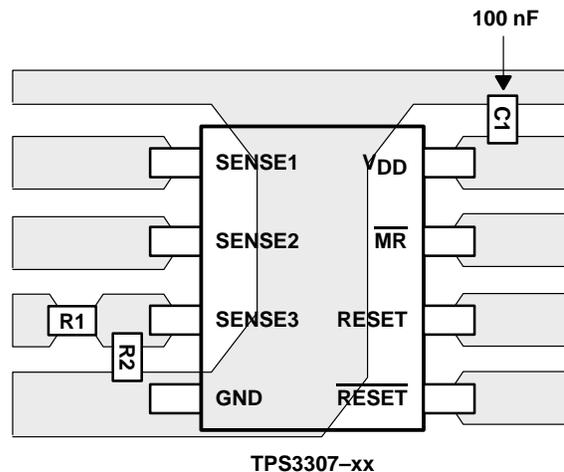
**Figure 29. Suggested Layout for a Circuit With the TPS3307-xx**
