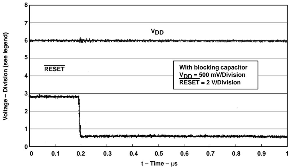
Figure 31.  $V_{DD}$  - Line of TPS3306-33 With a Capacitor and 100-k $\Omega$  Pullup Resistor at the  $\overline{RESET}$  Output
