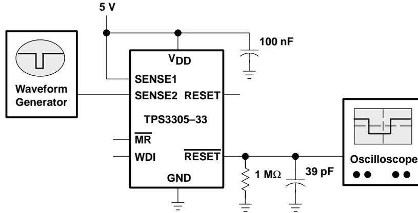
**Figure 13. Circuit for Measuring Breakdown Voltage Over Pulse Width**
