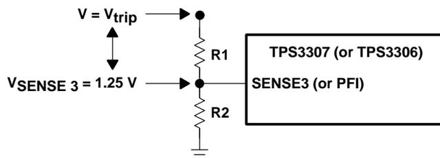
**Figure 12. Trip-Point Voltage**
