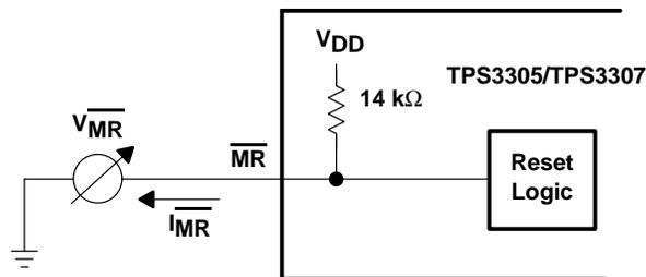
Figure 20. Internal Structure of the  $\overline{\text{MR}}$  Circuit
