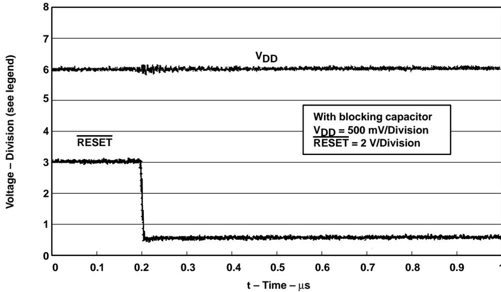
Figure 30.  $V_{DD}$  - Line of TPS3305-33 With a Capacitor
