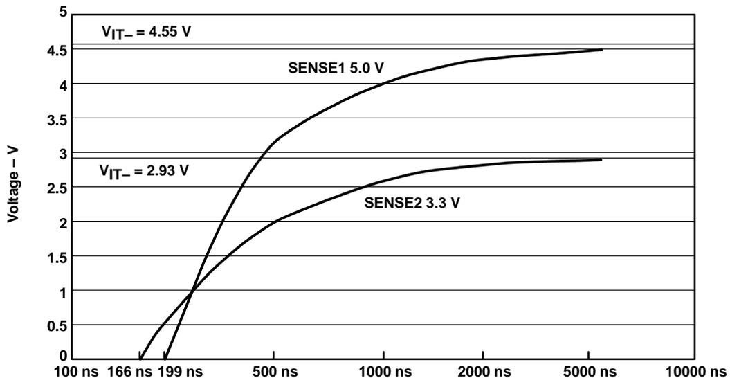
**Figure 14. Breakdown Voltage Over Pulse Width (TPS3305-33, TPS3307-33)**
