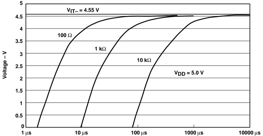
Figure 17. Breakdown Voltage Over Pulse Width With a Low-Pass Filter at SENSE1
