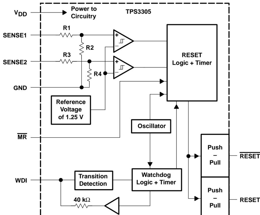
**Figure 4. Block Diagram of the TPS3305**
