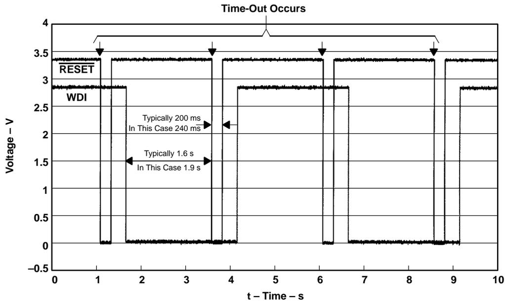
Figure 22. Watchdog Measurement 1 – Time-Out
