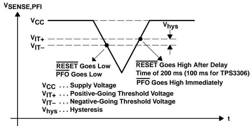
**Figure 9.  $V_{IT+}$ ,  $V_{IT-}$ , and  $V_{hys}$  Timing Relationships**
