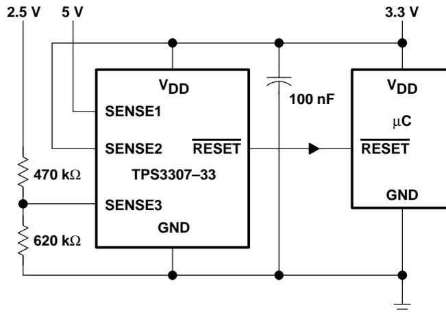
**Figure 27. Supervising 2.5-V, 3.3-V, and 5-V Supplies With One Device**
