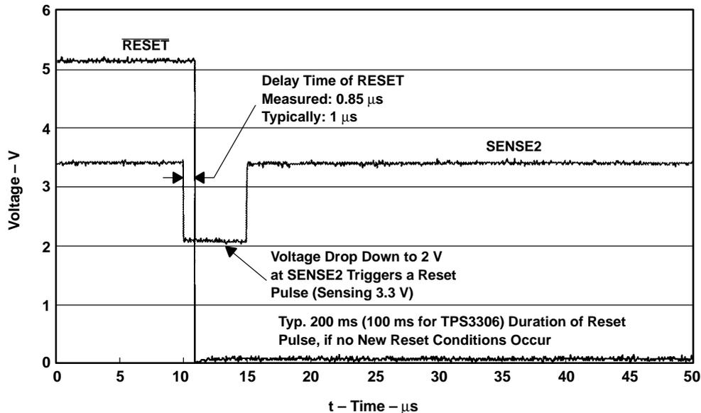
**Figure 11. Measurement of the Voltage Drop at SENSE2 Input**
