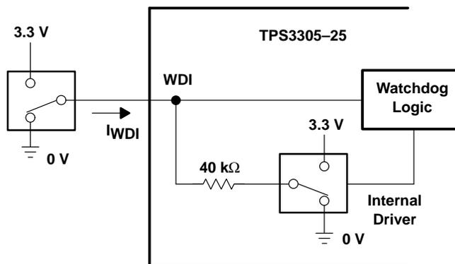
**Figure 25. Internal Structure of the Watchdog Autoreset Driver**
