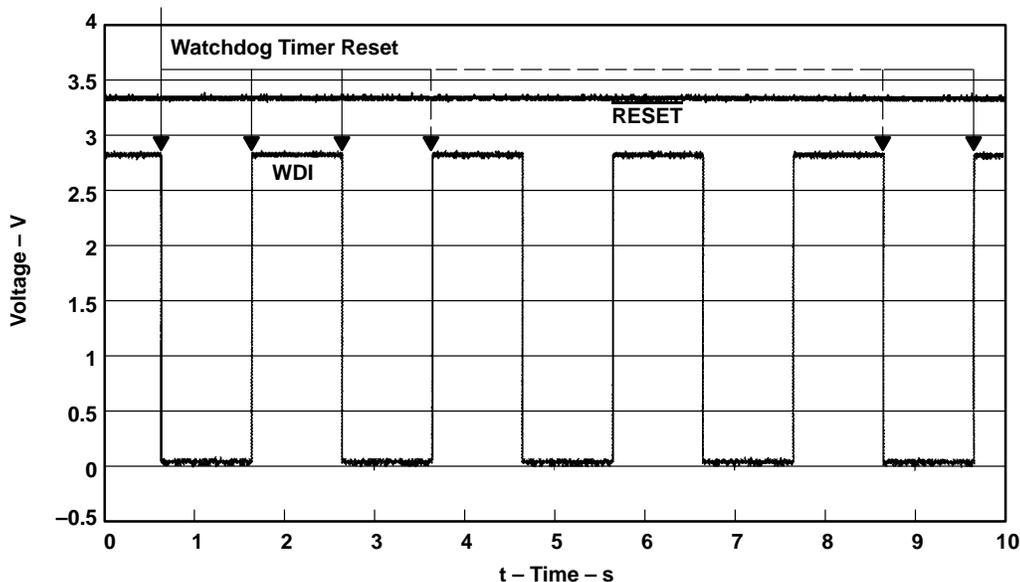
Figure 23. Watchdog Measurement 2 – No Time-Out
