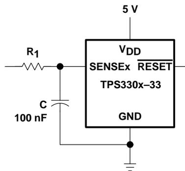
Figure 16. TPS330x With a Low-Pass Filter at SENSE Input
