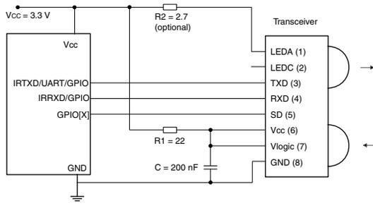
Figure 2. General Interfacing Block Diagram for IrDA and RC
