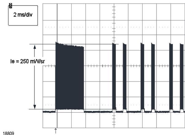
Figure 9. Signal from the IR transmitter with new Alkaline batteries. The measured intensity is constant.
