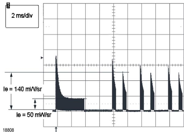
Figure 8. Signal from the IR transmitter with empty batteries. The measured intensity is decreasing during the burst.
