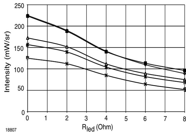
Figure 6. Current-limiting resistor vs. on-axis intensity for TFDU6102 (five randomly selected transceivers). Applied operating voltage  $V_2 = 3.3$  V
