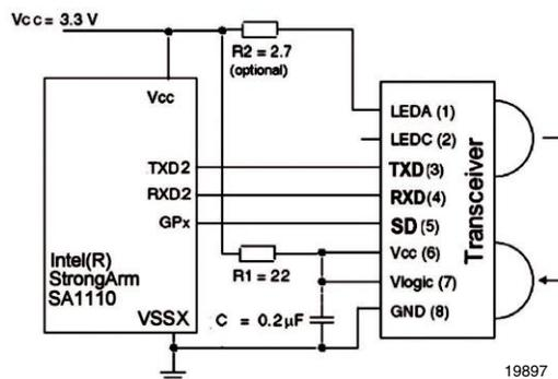
Figure 16. Intel SA-1110 Processor, StrongArm, in IrDA/RC applications
