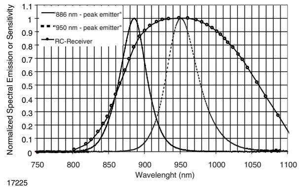
Figure 4. Spectral sensitivity and emitter „Overlap“
