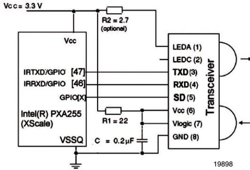
Figure 17. Intel PXA255 Processor, Xscale, in IrDA/RC applications
