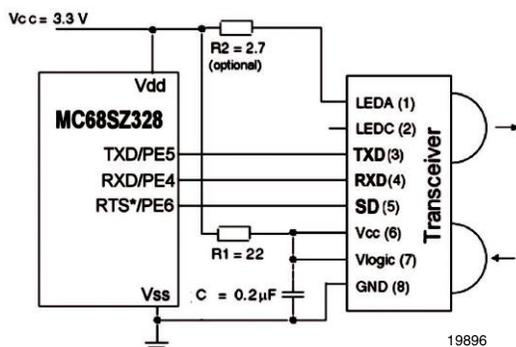
Figure 15. Motorola MC68SZ328 Processor, DragonBall, interfaced for IrDA/RC applications
