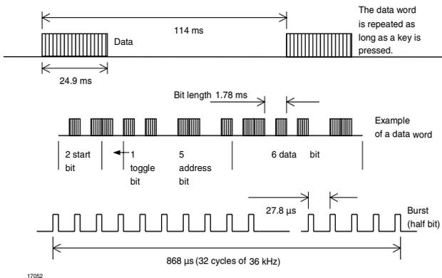
Figure 14. Philips RC5 IR remote control protocol
