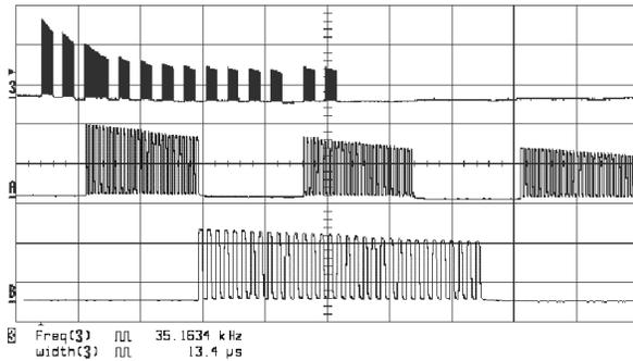
Figure 13. RC5 optical signals of Key '3'
