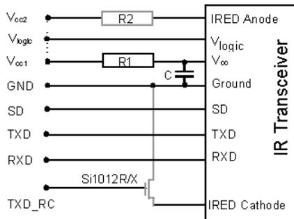
Figure 3. General Interfacing Block Diagram for IrDA<sup>®</sup> and RC using an n-channel FET when only a separate RC port is available.
