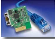
This board is populated with the 28-pin ENC28J60 Ethernet controller which interfaces to the RJ-45 connector. It can be plugged into the Explorer 16 development board (DM240001), allowing connection to any of Microchip's 16- and 32-bit products when used in conjunction with the free Microchip TCP/IP stack.
