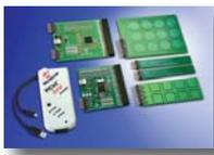
Includes two main boards: one populated with a PIC16F72X 8-bit MCU and the other with a PIC24F256GB110 16-bit MCU; and four daughter boards for developing keys, sliders and a matrix.
