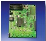
This development board provides a low-cost, highly configurable development system for Microchip's line of extreme low power 16-bit PIC24F microcontrollers featuring sleep currents down to 20 nA. The board supports development on PIC24F16KA102, PIC24FJ64GA102 and PIC24F64GB002 families of MCUs. This board can be powered by more than five sources including batteries and energy harvesting modules and supports a variety of common components that can be selectively enabled.
