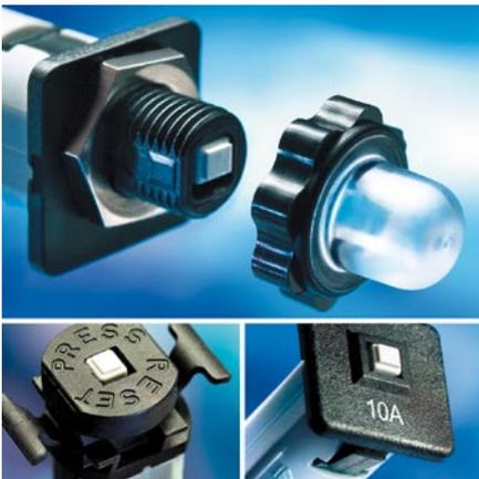
Thermal circuit breakers for equipment have the advantage that they are insensitive to inrush currents that occur when switching on motors and transformers. However, dimensioning of the rated current is not only determined from the rated current of the load. Other parameters such as in-rush current, overloading capacity, operating duty and ambient temperature should also be taken into consideration.
