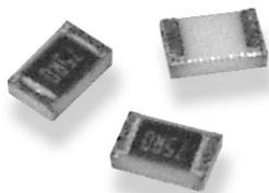
The RN73 series is a high stability precision chip resistor range offering various power dissipations relating to chip size, TCR's down to 5ppm/°C and resistance tolerances to 0.1%. The resistor is produced with three sputtered layers giving optimum performance. Values are restricted to the E96 and E24 value grids. The RN73 has accurate and uniform physical dimensions to facilitate placement.
