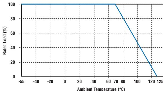
For temperatures in excess of 70°C the load shall be derated in accordance with this curve.
