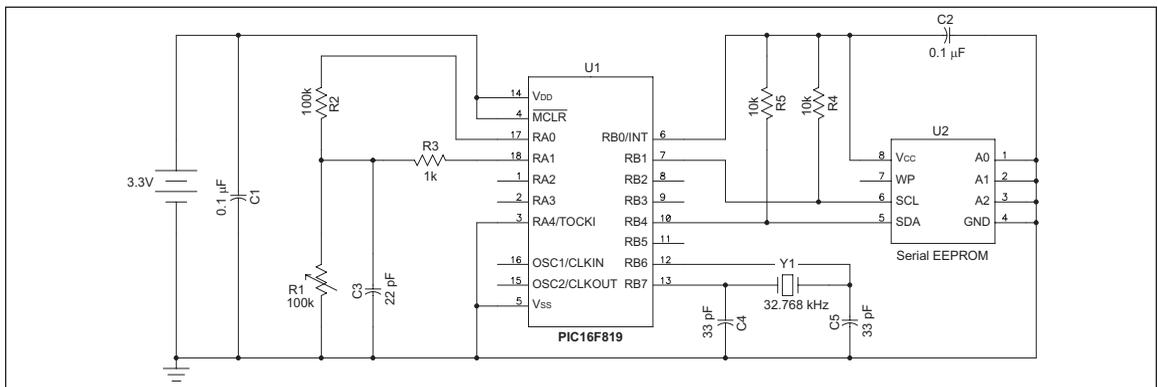
In Figure 1-2, I/O pins are used to power the EEPROM and the sensor. Many PIC MCU devices can source up to 20 mA of current from each I/O, so there is no need to provide additional components to switch the power.
