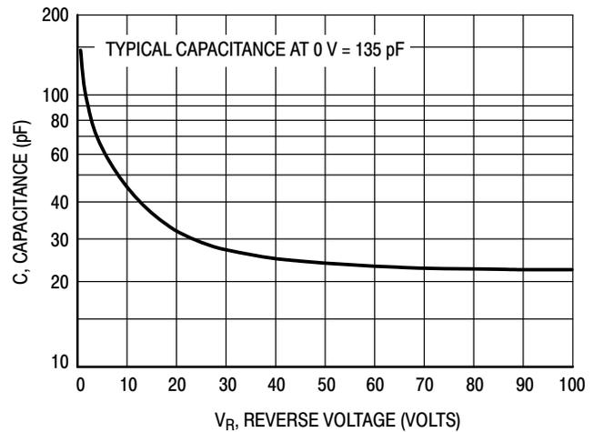
Figure 5. Typical Capacitance
