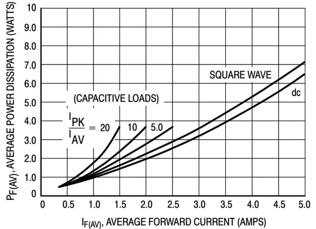
Figure 8. Power Dissipation
