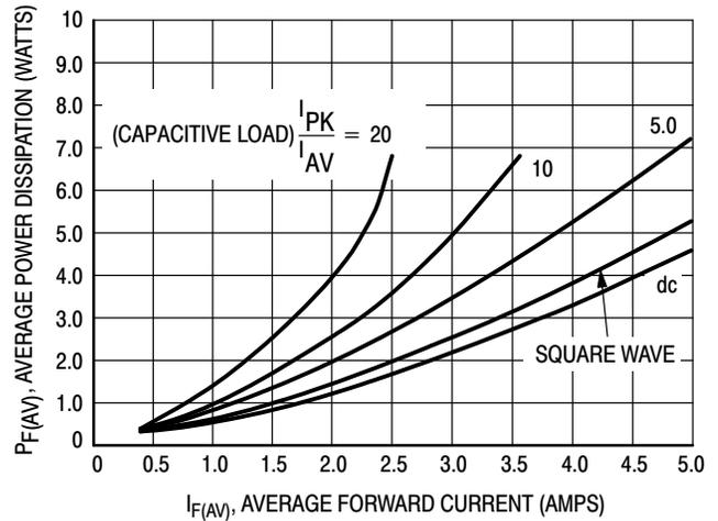
Figure 3. Power Dissipation
