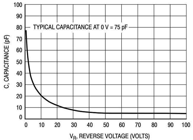
Figure 10. Typical Capacitance
