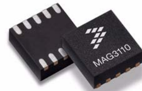
10-PIN DFN 2 mm x 2 mm x 0.85 mm CASE 2154-02
