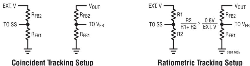
Figure 5(b): Setup for Ratiometric and Coincident Tracking
