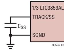
Figure 6. Using the TRACK/SS Pin to Program Soft-Start
