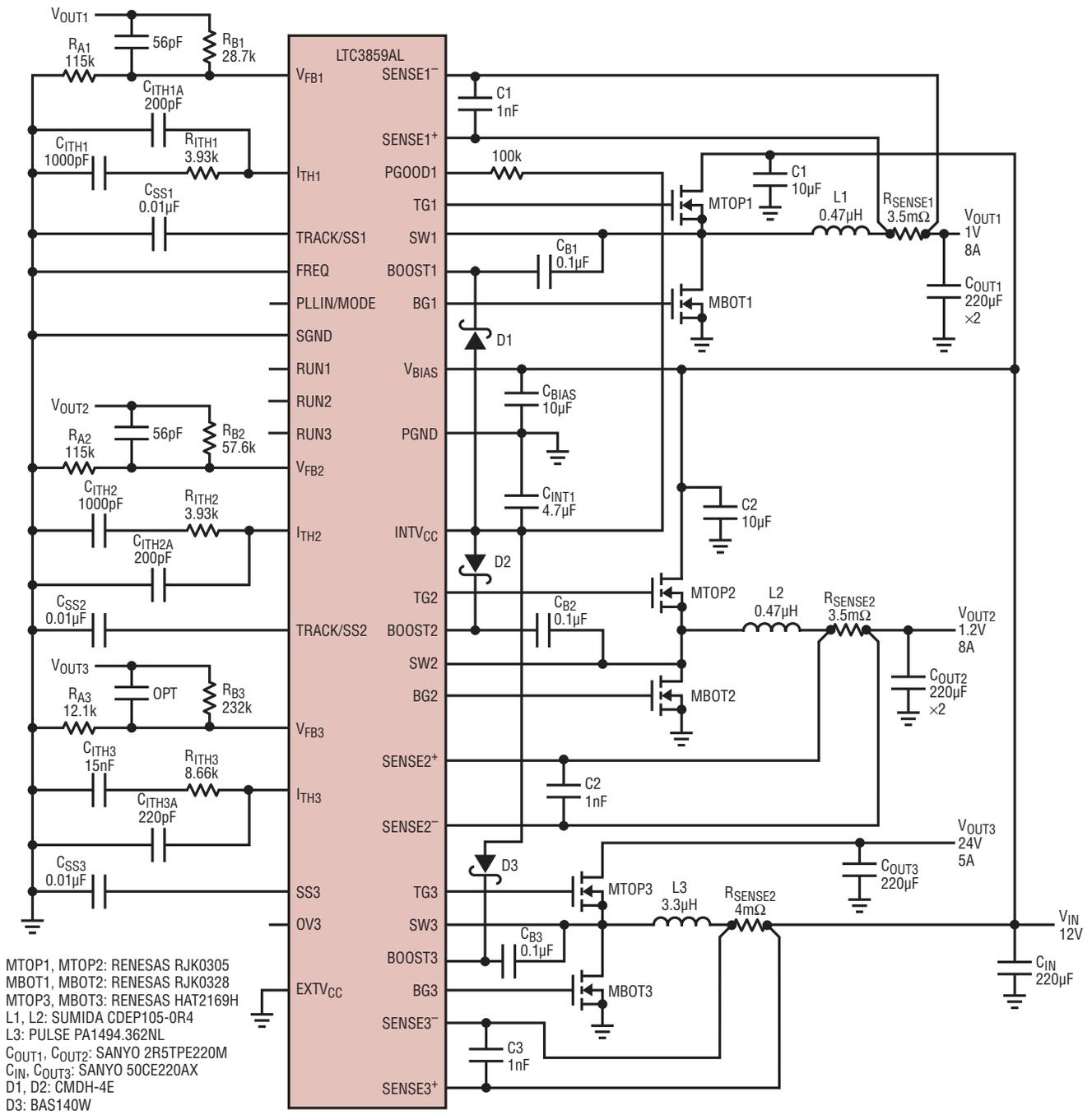
Figure 14. High Efficiency Triple 24V/1V/1.2V Converter from 12V V<sub>IN</sub>
