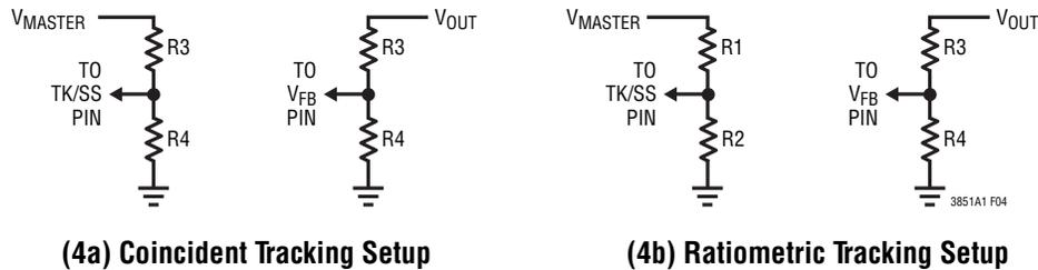
Figure 4. Setup for Coincident and Ratiometric Tracking
