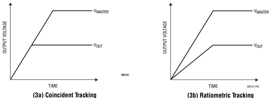
Figure 3. Two Different Modes of Output Voltage Tracking
