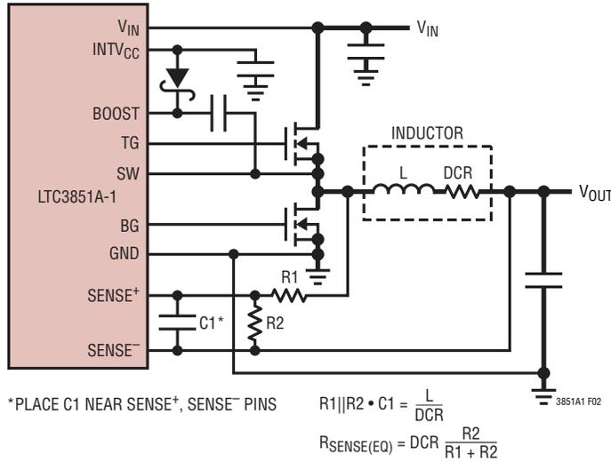
Figure 2. Current Mode Control Using the Inductor DCR
