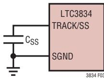
Figure 3. Using the TRACK/SS Pin to Program Soft-Start
