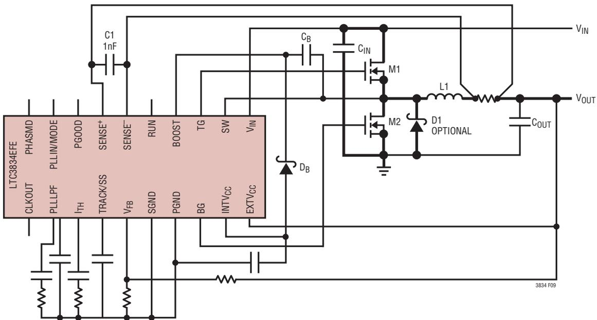
Figure 9. LTC3834 Recommended Printed Circuit Layout Diagram
