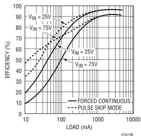
Figure 6. Efficiency in Pulse-Skip/Forced Continuous Modes
