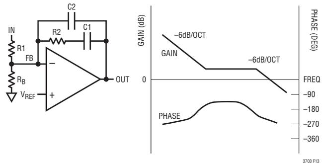
Figure 13. Type 2 Schematic and Transfer Function
