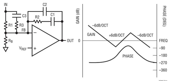
Figure 14. Type 3 Schematic and Transfer Function
