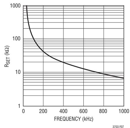
Figure 7. Timing Resistor ( $R_{SET}$ ) Value
