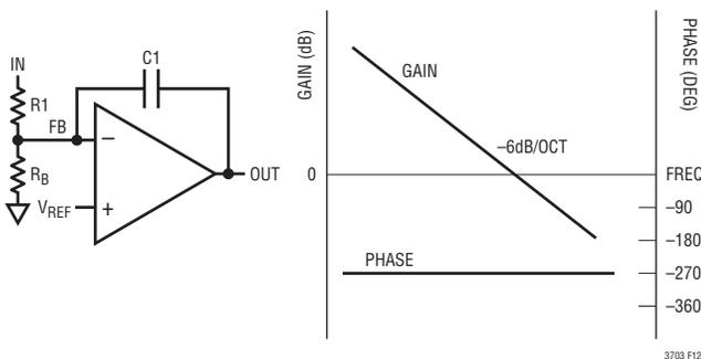
Figure 12. Type 1 Schematic and Transfer Function
