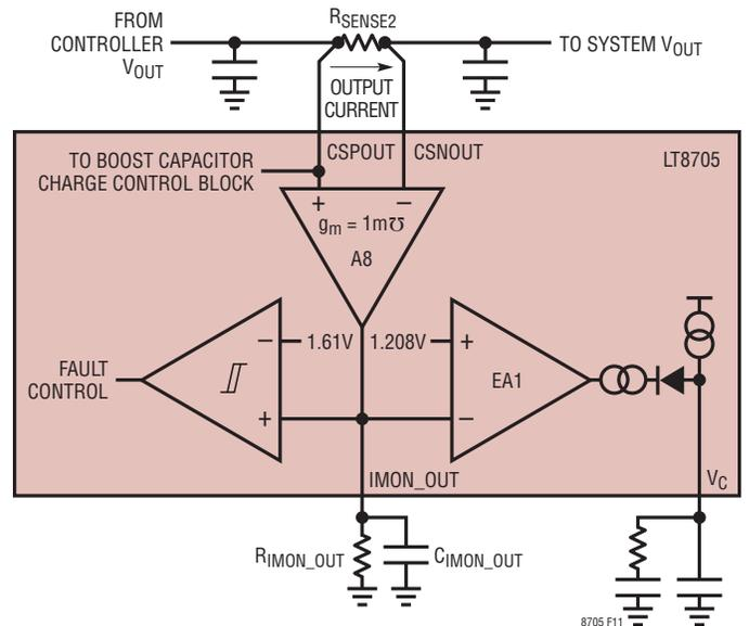
Figure 11. Output Current Monitor and Limit
