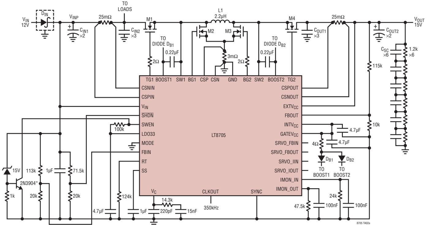
C<sub>IN1</sub>, C<sub>OUT2</sub>: 100μF 20V SANYO OS-CON 205A100M
