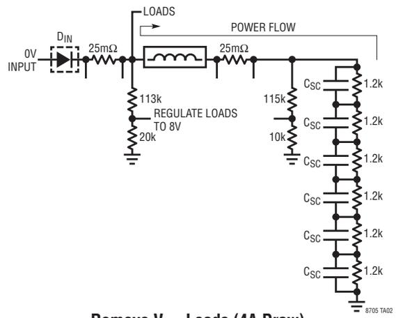
**Remove V<sub>IN</sub>. Loads (4A Draw) Regulated to 8V from Supercaps**
