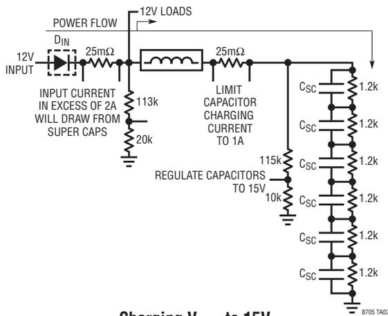
**Charging V<sub>OUT</sub> to 15V with 1A Current**
