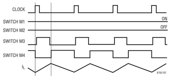
Figure 7. Boost Region ( $V_{IN} \ll V_{OUT}$ )
