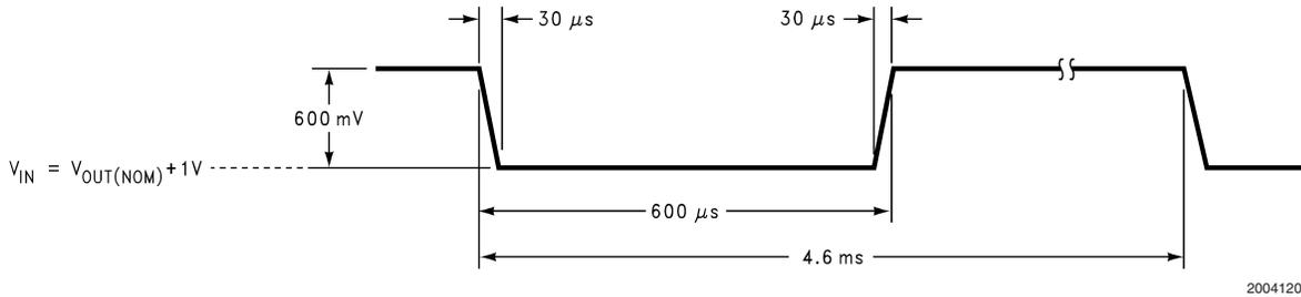
FIGURE 2. Figure 2. Line Transient Input Test Signal.
