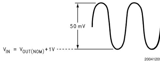
FIGURE 3. Figure 3. PSRR Input Test Signal.
