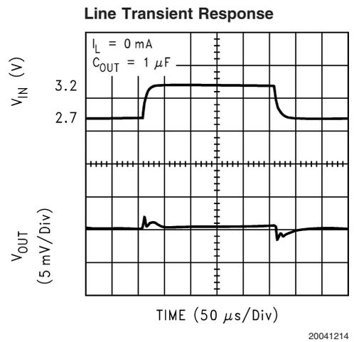
**Typical Performance Characteristics.** Unless otherwise specified,  $C_{IN} = C_{OUT} = 1.0 \mu\text{F}$  Ceramic,  $V_{IN} = 2.8\text{V}$ ,  $T_A = 25^\circ\text{C}$ , Shutdown pin is tied to  $V_{IN}$ . (Continued)
