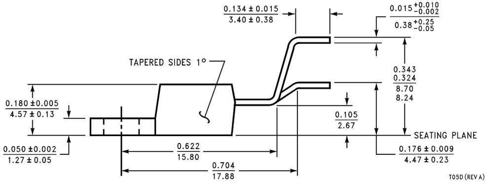
**TO220 5-lead, Molded, Stagger Bend Package (TO220-5)**
