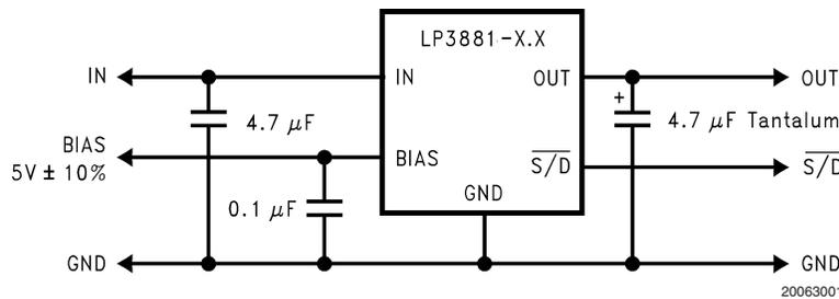
At least 4.7 μF of input and output capacitance is required for stability.
