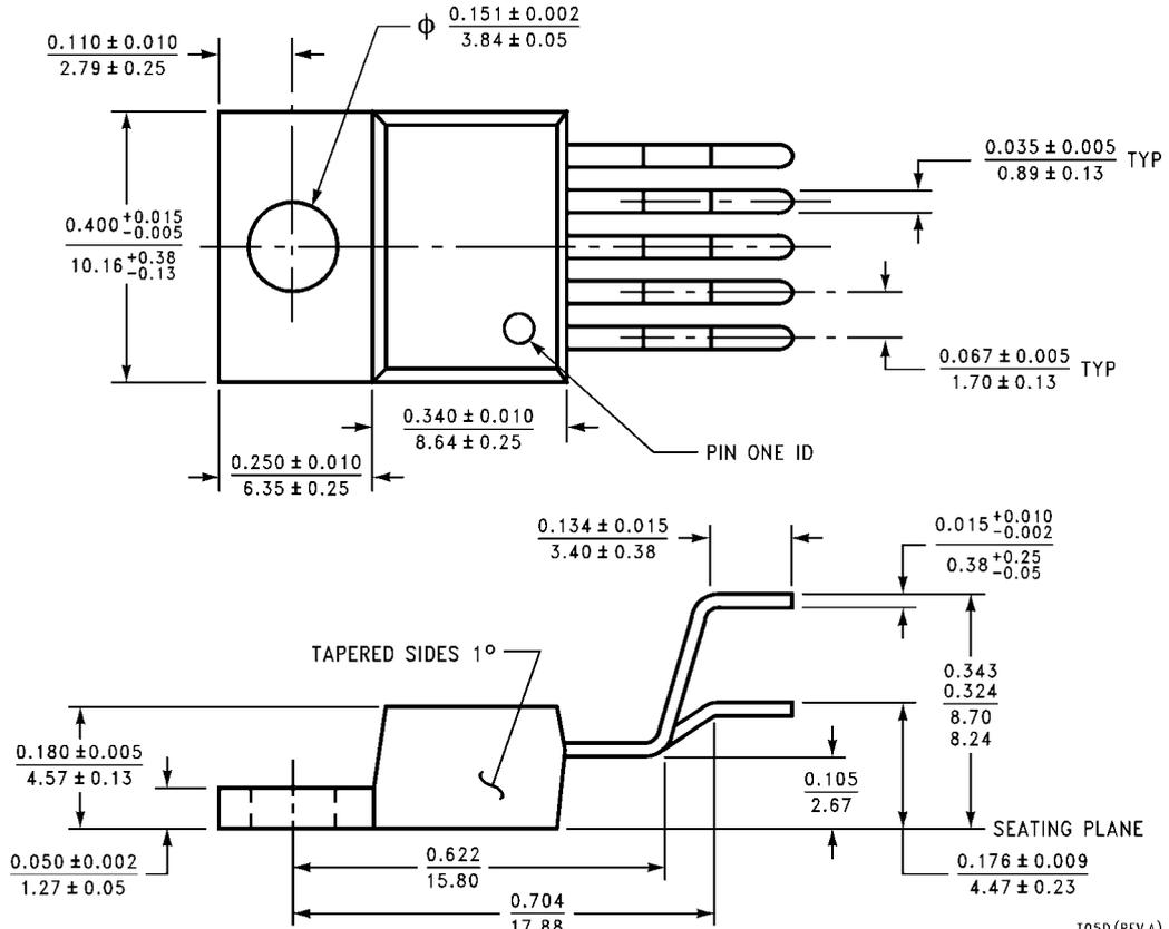
**TO220 5-lead, Molded, Stagger Bend Package (TO220-5)
