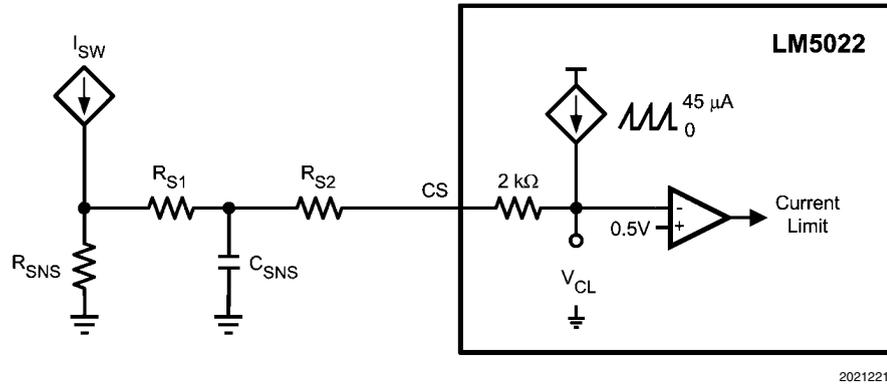
FIGURE 4. Slope Compensation
