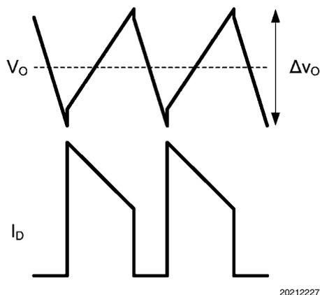
FIGURE 6.  $\Delta V_O$  Using Low ESR Capacitors
