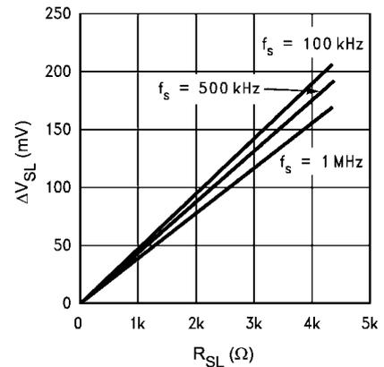
FIGURE 5. External Slope Compensation  $\Delta V_{SL}$  vs  $R_{SL}$
