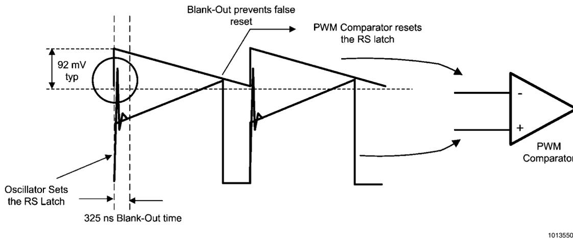
**FIGURE 2. Basic Operation of the PWM Comparator**
