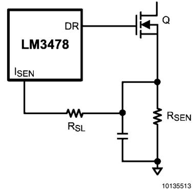
FIGURE 4. Adding External Slope Compensation
