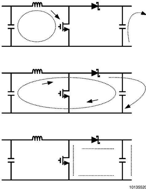
FIGURE 12. Current Flow In A Boost Application
