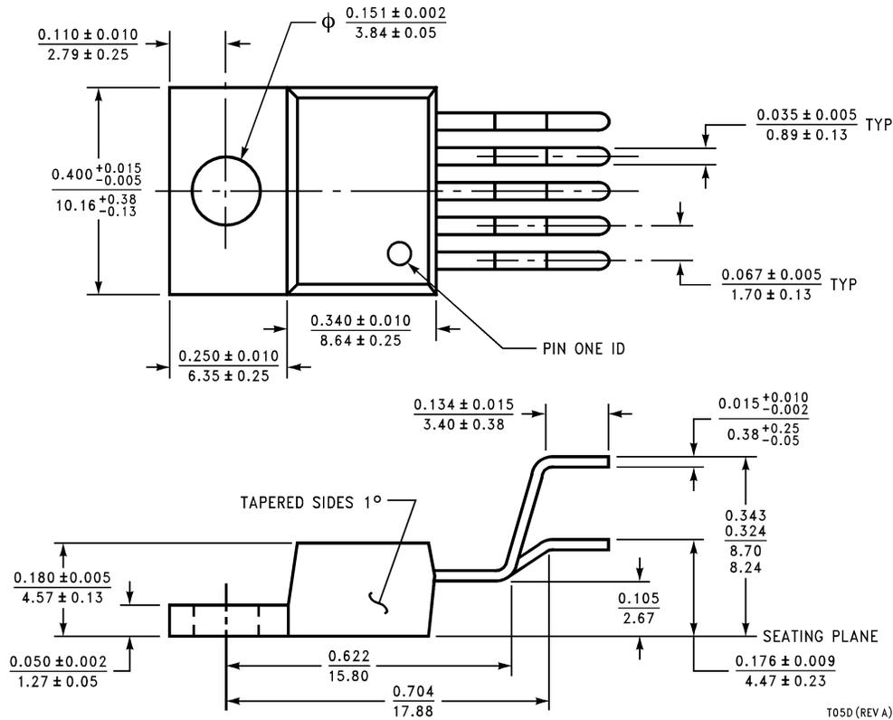
**Bent, Staggered 5-Lead TO-220 (T)**
