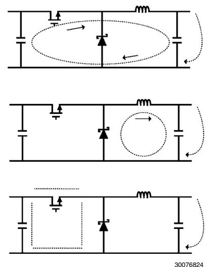
**FIGURE 6. Current Flow in a Buck Application**
