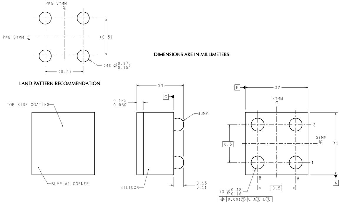
**4-Bump Thin micro SMD Ball Grid Array Package (Small Bump)**
