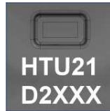
Laser marking on HTU21D sensor
