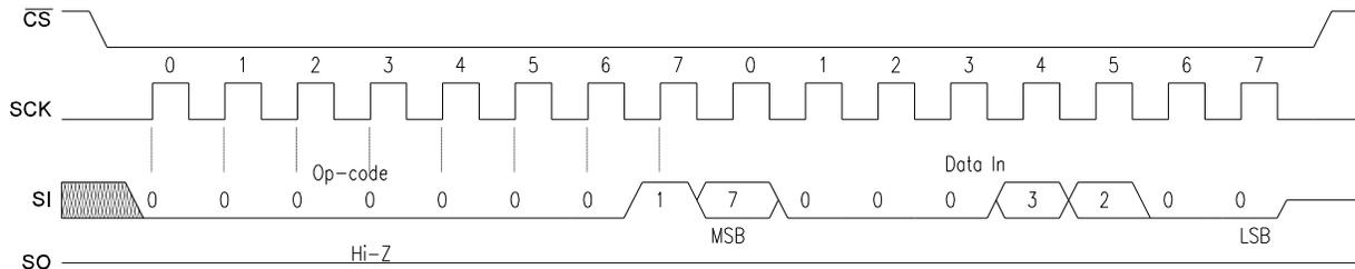
**Figure 8. WRSR Bus Configuration (WREN not shown)**
