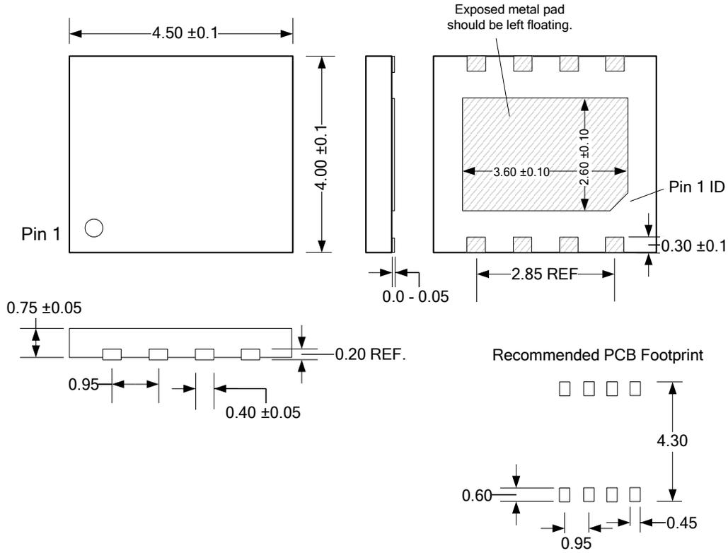
Note: All dimensions in millimeters. The exposed pad should be left floating.
