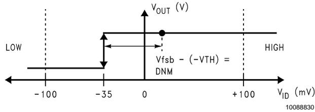
FIGURE 6. VTC of the DS90LV048A LVDS Receiver
