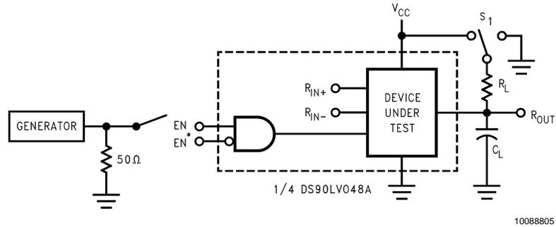
$C_L$  includes load and test jig capacitance.
