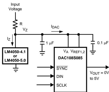
Figure 9. The LM4050 as a power supply
