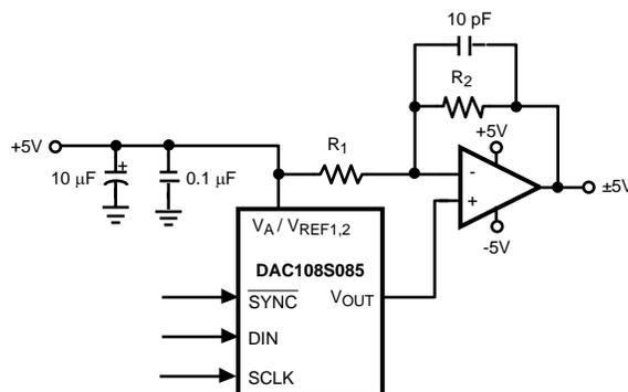
Figure 12. Bipolar Operation
