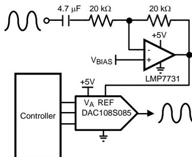
Figure 16. Programmable Attenuator
