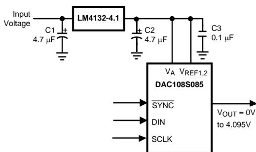
Figure 8. The LM4132 as a power supply
