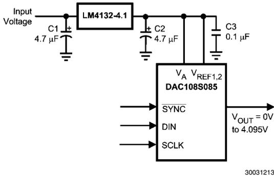
**FIGURE 8. The LM4132 as a power supply**
