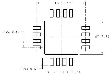
DIMENSIONS ARE IN MILLIMETERS
