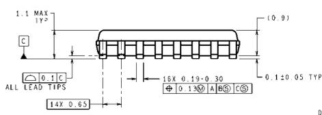
DIMENSIONS ARE IN MILLIMETERS
