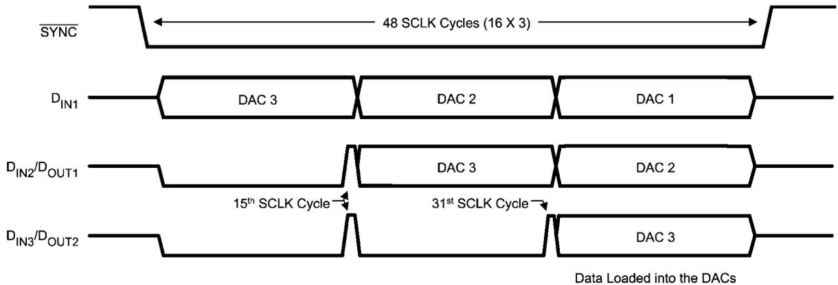
**FIGURE 7. Daisy Chain Timing Diagram**
