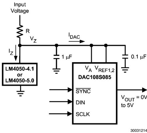
**FIGURE 9. The LM4050 as a power supply**
