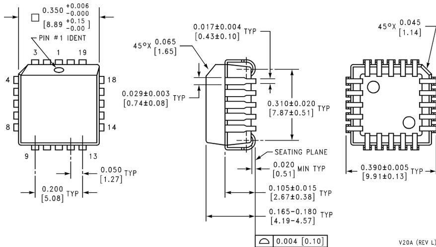
**Molded Chip Carrier (V)
