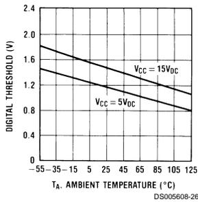
Digital Input Threshold vs. V<sub>CC</sub>
