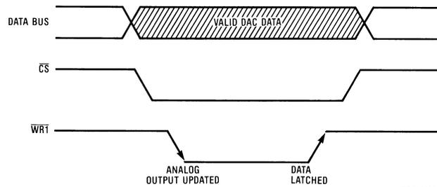
ILE=LOGIC "1";  $\overline{WR2}$  and  $\overline{XFER}$  GROUNDED
