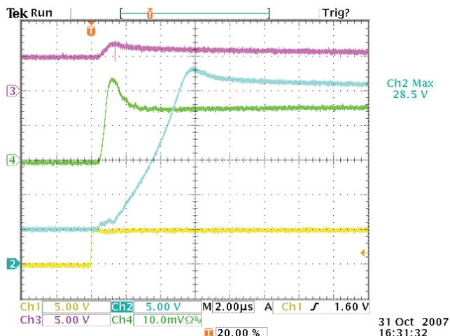
**Figure 19. Vin From 5 V to 60 V, 2- $\mu$ s Time Scale Zoom in Detail, CH2 5 V/div**
