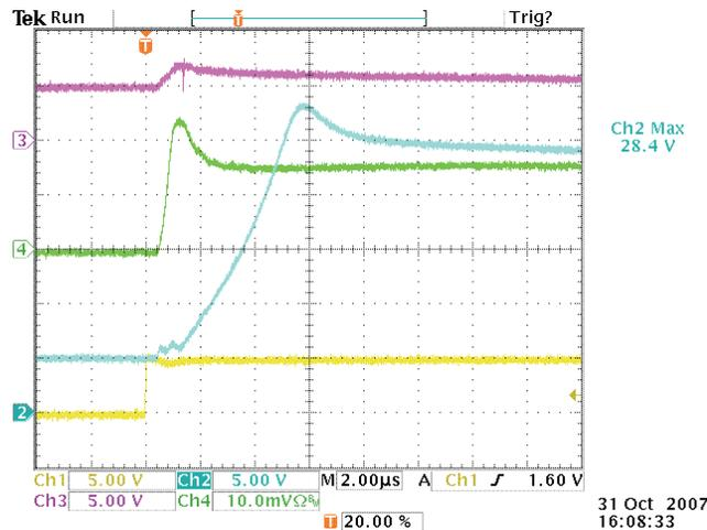
Figure 10. Vin From 5 V to 60 V, 2-μs Time Scale Zoom in Detail, CH2 5 V/div
