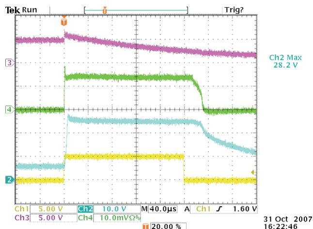
Figure 12. Vin From 5 V to 35 V
