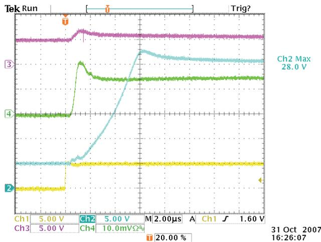
Figure 15. Vin From 5 V to 45 V, 2-μs Time Scale Zoom in Detail, CH2 5 V/div
