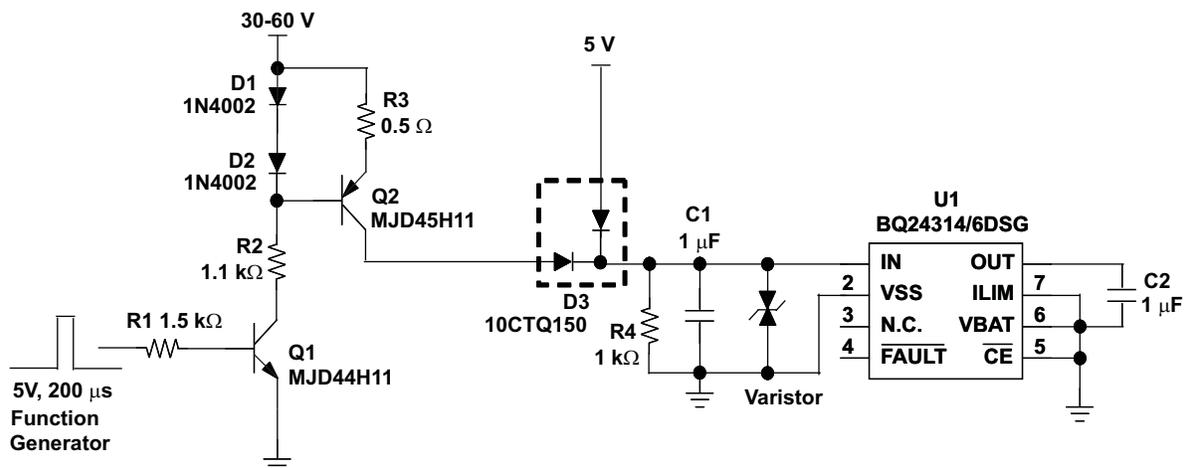
Figure 1. High-Voltage Pulse Transient Test Schematic
