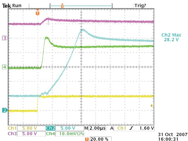
Figure 6. Vin From 5 V to 45 V, 2-μs Time Scale Zoom in Detail, CH2 5 V/div
