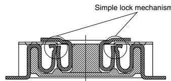
5. The lower connector bottom surface construction prevents contact and shorts between the PCB and metal terminals. Benefits include freedom in pattern wiring, helping to make PCB's smaller.
