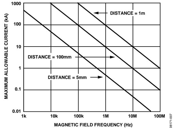
Figure 7. Maximum Allowable Current for Various Current-to-ADuM4160 Spacings
