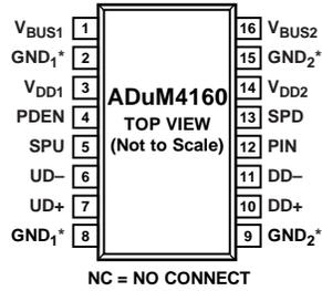
\*PIN 2 AND PIN 8 ARE INTERNALLY CONNECTED, AND CONNECTING BOTH TO GND<sub>1</sub> IS RECOMMENDED. PIN 9 AND PIN 15 ARE INTERNALLY CONNECTED, AND CONNECTING BOTH TO GND<sub>2</sub> IS RECOMMENDED.
