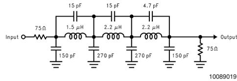
**FIGURE 9. 11 MHz Low Pass filter to eliminate harmonics at the signal input.
