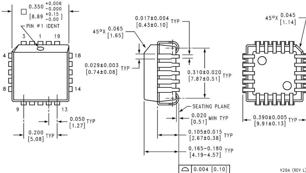
**Molded Chip Carrier Package (V)**
