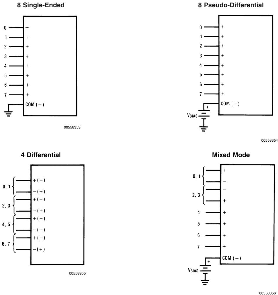
**FIGURE 1. Analog Input Multiplexer Options for the ADC0838**
