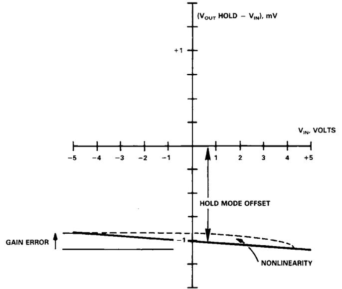
Figure 3. Hold Mode Offset, Gain Error and Nonlinearity
