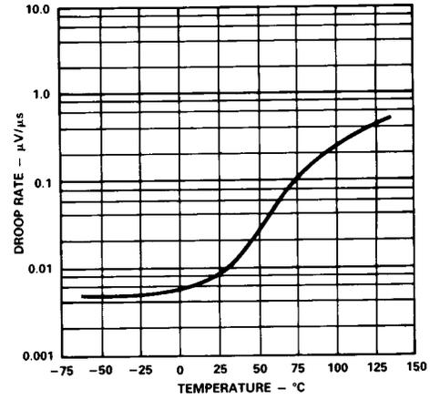
Droop Rate vs. Temperature,  $V_{IN} = 0\text{ V}$
