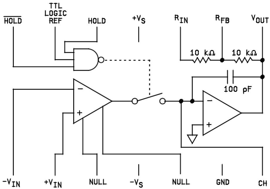
FIGURE 2. Block diagram.
