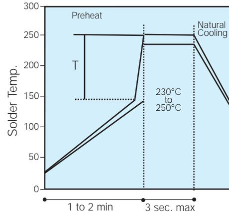
(Preheat chips before soldering)
